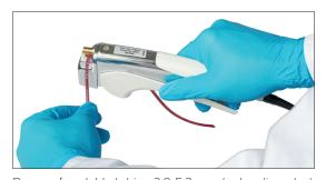
Range of sealable tubing 3.0-5.2 mm (outer diameter)
