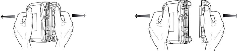
**NOTE:** The door can be immersed. Clean it separately with running water.
