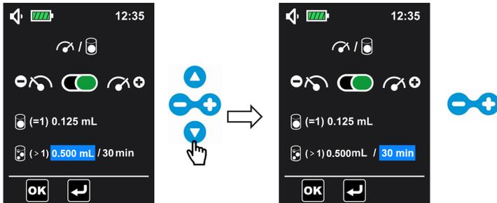
**NOTE:** Air in line alarm will be triggered when the detected cumulated bubbles volume is  $\geq$  to the customized volume value throughout the customized duration. The adjustment range of cumulated volume is from 0.25 mL to 0.75 mL by step of 0.125 mL, the adjustment range of time is 1 min, 5 min, 10 min, 15 min, 20 min, 25 min, 30 min (cumulated bubbles volume setting is 0.5 mL / 30 min by default).
