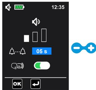
**NOTE:** Time between 2 alarm sounds can be adjusted from 3 seconds to 15 seconds with step of 1 second . This adjustment can modify the perception of an alarm. On this screen, the time between 2 alarm sounds is 5 seconds (by default).
