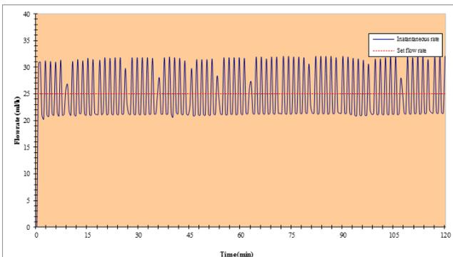
Start up and instantaneous at intermediate flow rate (25 mL/h, during first 2 hours of the set change interval, 24 hours)
