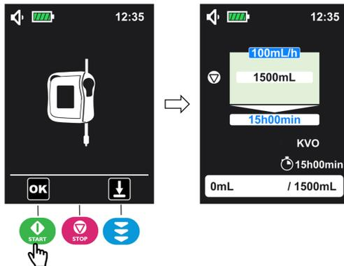
**Note:** Automatic priming can be stopped at any time by pressing the key. Once it is stopped, it is possible to continue priming by using *Semi-automatic priming* on page 31.
