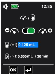
**NOTE:** Air in line alarm will be triggered when the detected single bubble volume is  $\geq$  to the customized volume value. The single bubble setting can be adjusted from 0.125 mL to 0.75 mL, with step of 0.125 mL (default setting: 0.125 mL).
