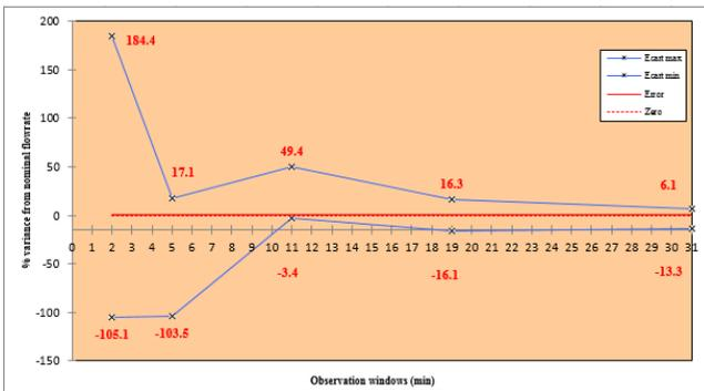
Trumpet curves for 2, 5, 11, 19, 31 minute observation windows (1 mL/h, during last hour of the set change interval, 24 hours)
