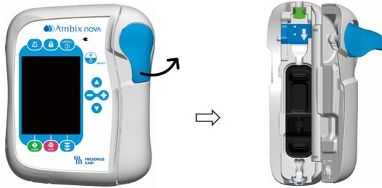
2. Align the set along with the tube guide of the pump with the right flow direction (the arrow mark on the pump indicates the direction of the flow).
