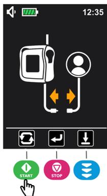
2. **Wait** until the progress bar has filled up and the pump stops priming automatically.
