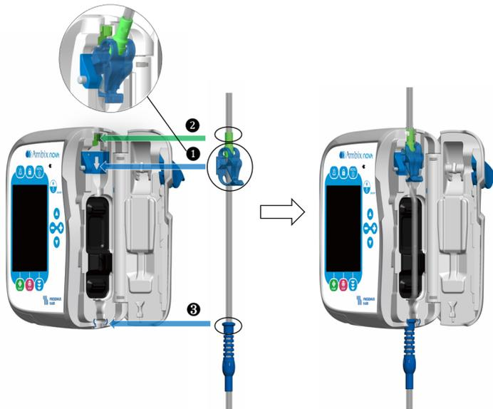
5. Close the pump door by pushing the door lever down .
