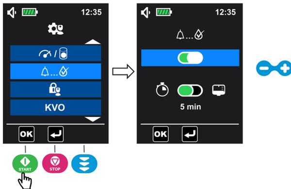
2. Once the pre-alarm is activated, press to go down to choose the mode to trigger the pre-alarm. Press to select remaining volume before end of infusion or press to select remaining time before end of infusion (activated by default).
