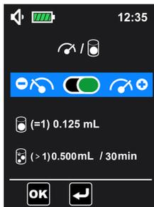
**NOTE:** Low level = an occlusion alarm will be triggered for a pressure value of  $487.5 \text{ mmHg} \pm 187.5 \text{ mmHg}$  in the administration set; High level = an occlusion alarm will be triggered for a pressure value of  $787.5 \text{ mmHg} \pm 262.5 \text{ mmHg}$  in the administration set.
